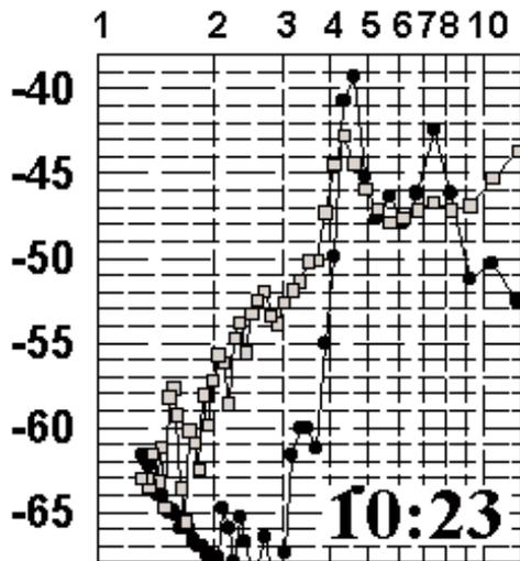
Figure 2. Mean RCS vs grazing angle for HH (gray) and VV (black)symbols shows larger HH echoes at the front.
