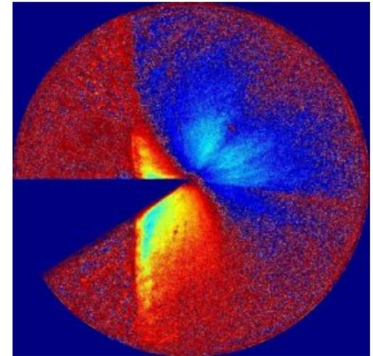
Radial velocity summed image, blue approaching and red receding. Here mean drift current of the wave field dominates the image. Comparisons with ADCP's in the area show good comparisons.
