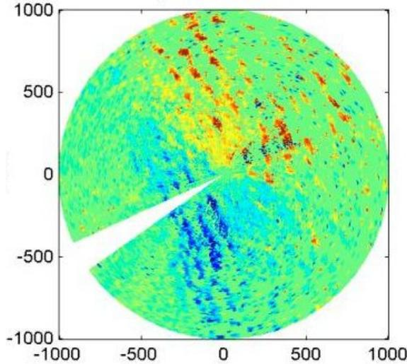
New Doppler image of radial velocity pattern of waves.
