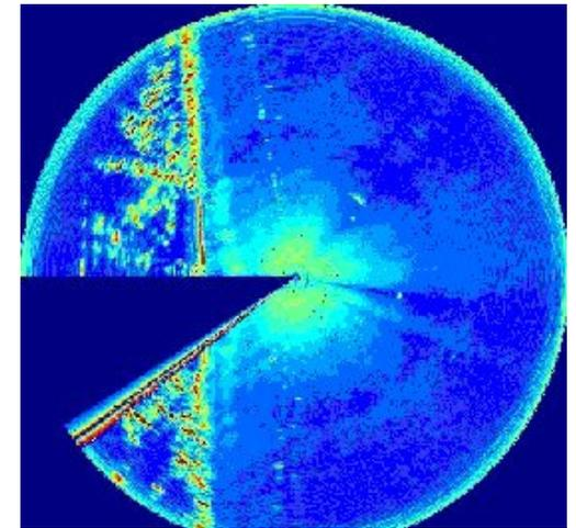
Intensity 512-rotation sum, ocean wave patterns averaging to a mean value. The nearshore bar can be mapped due to enhanced wave breaking
