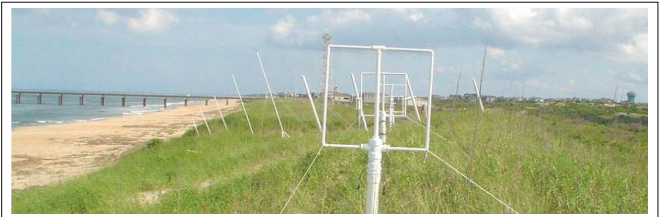
FIGURE 1: A photo is shown of a multi-frequency monostatic radar site at the US Army Corps of Engineers Field Research Facility, with a 4 loop-element receive array and a short log periodic transmit array
